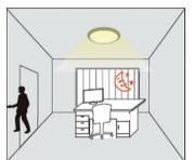
Once the step 1 function has run, the fitting will drop to the selected brightness for the selected period of time subject to no further movement.
