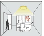
When movement is detected, the fitting will turn on and stay on for the selected period of time allocated via the remote control.
